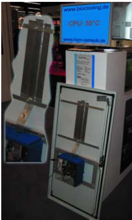
Figure 1: GraviTherm in a cabinet application
