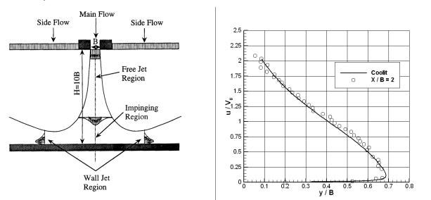
Fig. 1 (left) shows schematic of the experiment and Fig 2 shows velocity profile two jet-widths from axis.
