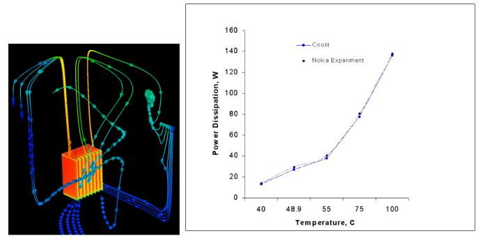
Flow pattern and predicted vs experiment power dissipation.
