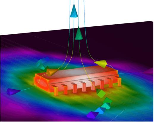
Coolit model of the Nokia board with SO16 device
