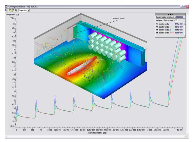
Coolit model of the power supply and temperature as a function of time at several monitor probe locations.
