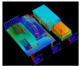
Redirecting more airflow towards the heat sink side of the assembly improved cooling.
