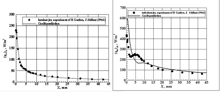
Left: Heat flux along the plate at Re=450. Right: Heat flux along the plate at Re= 2750.
