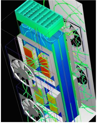
Coolit model of TEC-cooler for surgical blankets.
