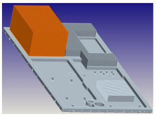
Removing least effective fins reduced heat sink weight.
