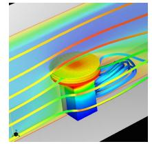
Coolit simulation on a Calgreg radial heat sink.
