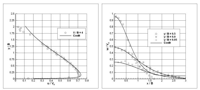
Fig 3. Velocity profile four jet-width from axis (left) and Fig. 4 shows y-velocity at several locations.
