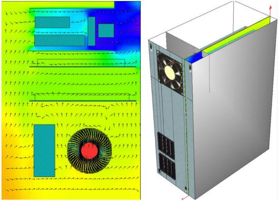
Coolit easily models complex curved surfaces such as this spiral heatsink.
