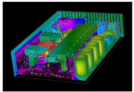
Coolit model of a rectifier unit.
