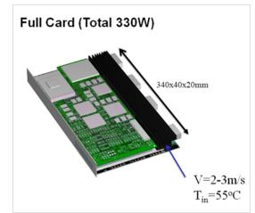
Heat pipe transfers heat from front of card to heat sink on the back.
