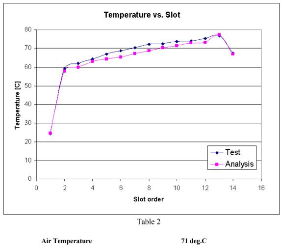
Predicted vs measured temperatures at different slots.
