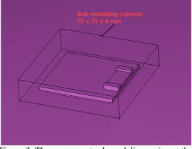
Figure 3: The component sub-modeling region at the main enclosure
