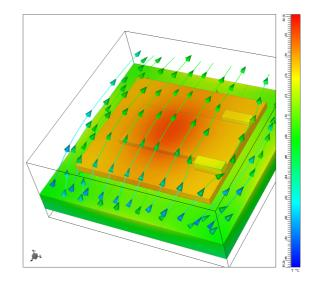
Figure 9: air velocity vector at the sub model from the main model B.C.
