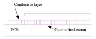
Figure 7: The component model cross section at a wire frame view.
