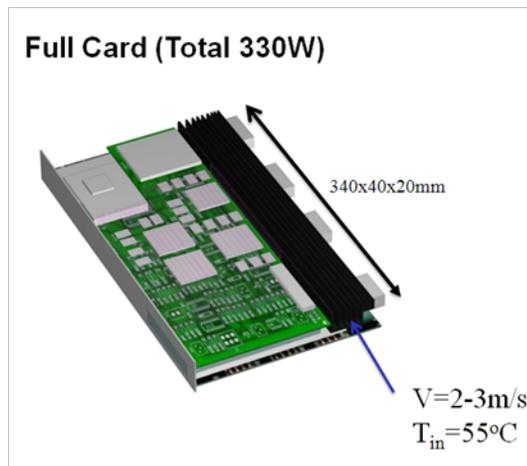
Heat pipe transfers heat from front of card to heat sink on the back.
