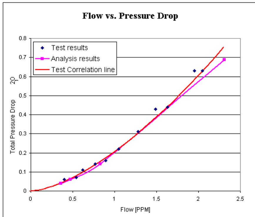
were plotted as a best fit curve (red solid line) and the results were compared with the Coolit predictions (magenta line). Excellent agreement was observed throughout the entire pressure-flow range.
