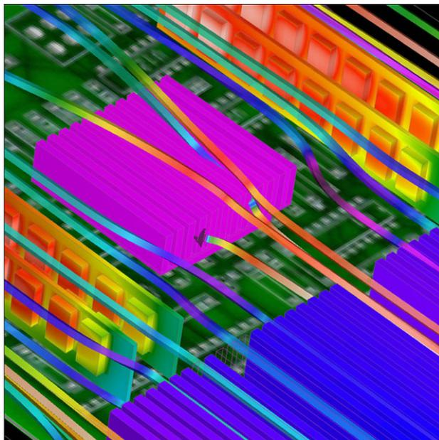
CoolitPCB model of a blade server board with stream rods painted in velocity magnitude.
