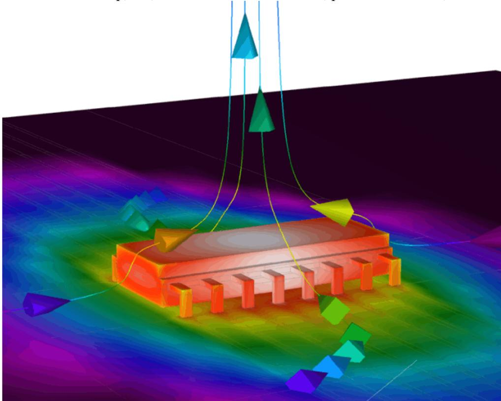
Coolit model of the Nokia board with SO16 device
