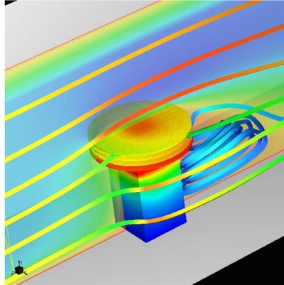
Coolit simulation on a Calgreg radial heat sink.
