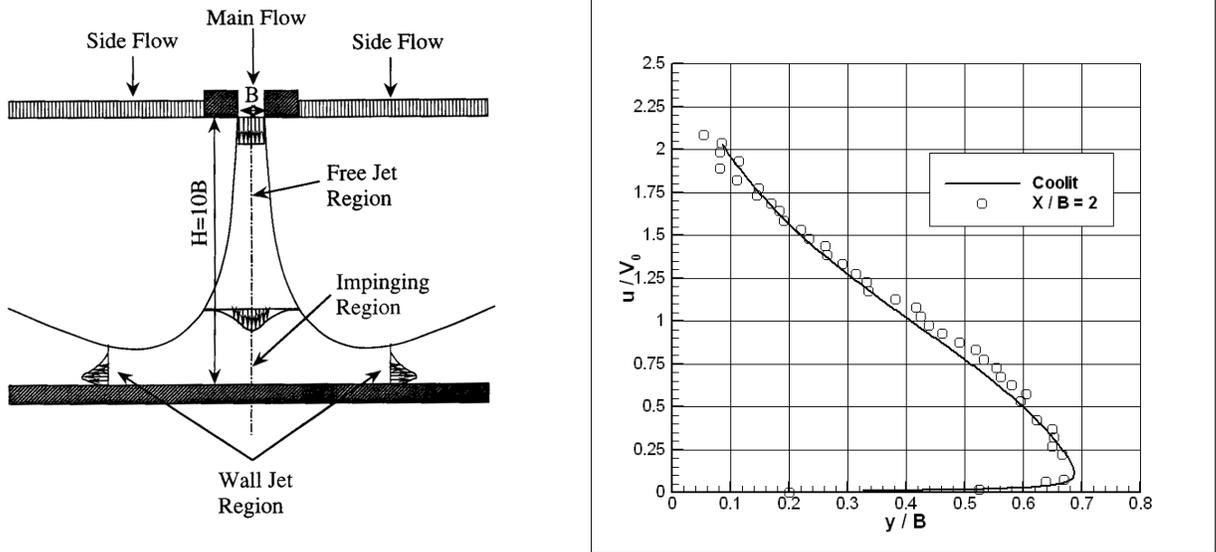
Fig. 1 (left) shows schematic of the experiment and Fig 2 shows velocity profile two jet-widths from axis.
