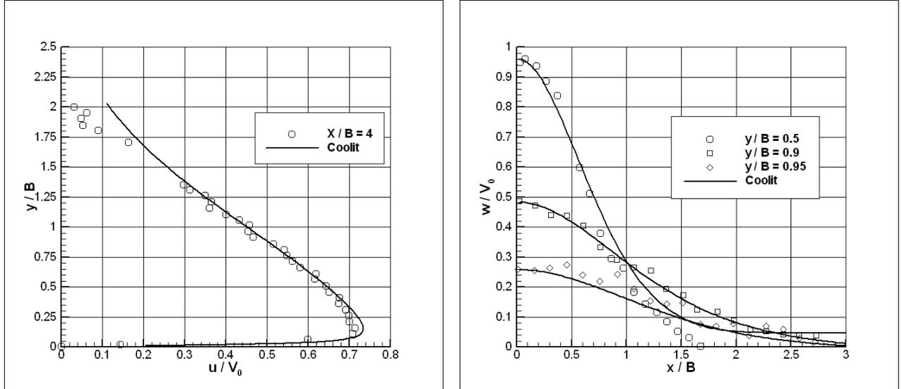
Fig 3. Velocity profile four jet-width from axis (left) and Fig. 4 shows y-velocity at several locations.
