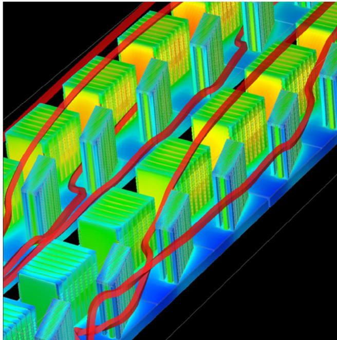
Coolit analysis shows that the tilted module design will deliver cool air to each module.
